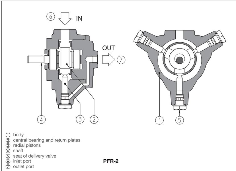
PFR are fixed displacement radial piston pumps with positive drive construction of the pistons ③ (without return spring) for high performance and low noise level.
